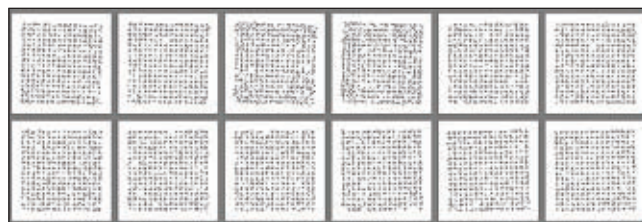
▲ Fig. 6 UL Constellations from each user terminal in indoor scenario 1 after ZF decoding. 14
