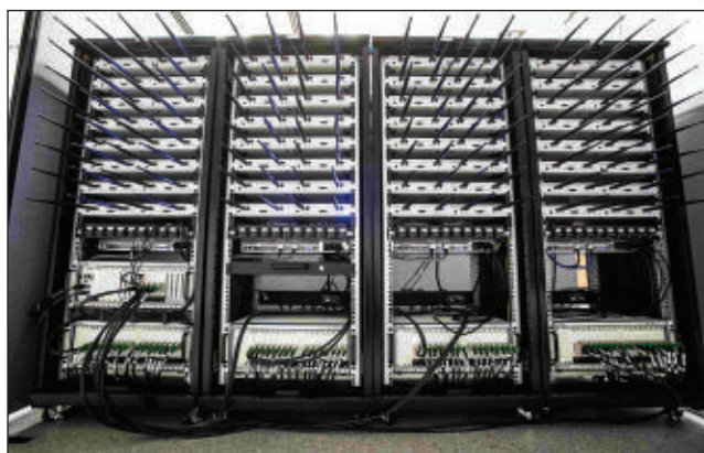
▲ Fig. 3 Bristol 128-antenna Massive MIMO testbed, which is managed by Bristol Is Open (BIO), a joint venture between the University of Bristol and the Bristol City Council.
