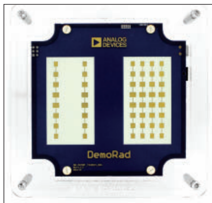
▲ Fig. 1 Demorad 24 GHz radar platform showing transmit (left) and receive (right) antennas.
