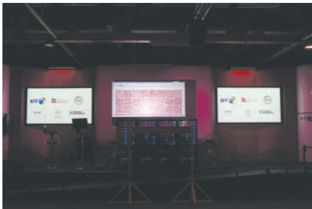
▲ Fig. 9 Bristol Massive MIMO testbed receiving 64-QAM from 24 user clients at Adastral Park (BT R&D).
